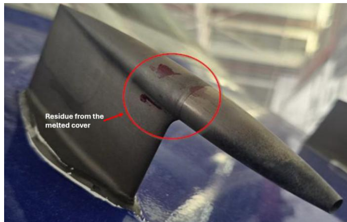
Figure 4: Residue from the pitot probe cover stuck on the RH pitot probe
